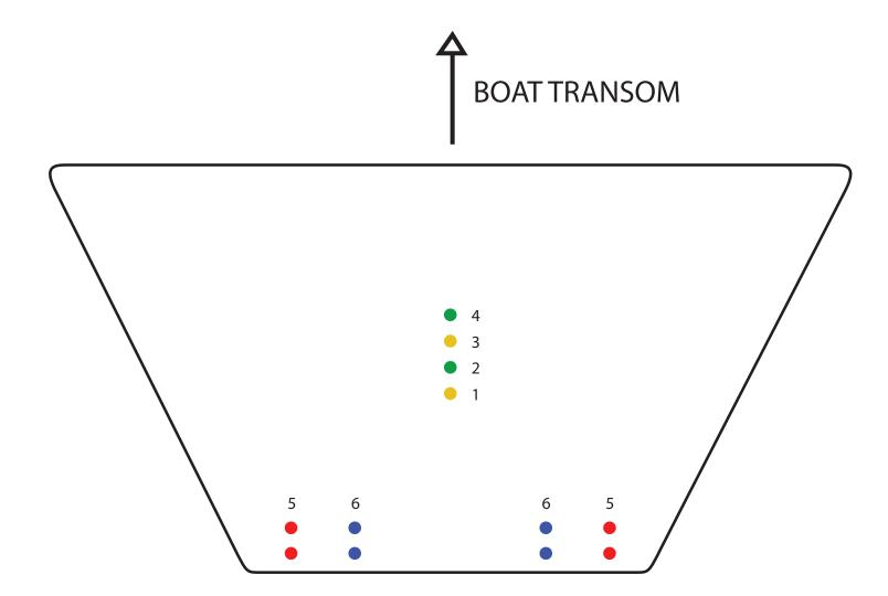
HOLES 1 AND 3 ARE FOR THE 21" DROP LADDERS HOLES 2 AND 4 ARE FOR THE 18" DROP LADDERS
