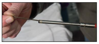
From the engine end of the cable carefully slide the braided cable into the cable housing.
