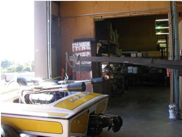
At this point the engine should be slightly raised at the rear. This will remove the weight off the snout of the pump.
