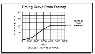
Figure 2 The Factory Equipped Curve.
