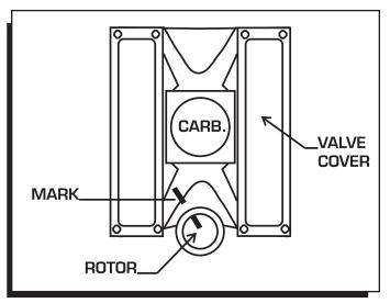
Figure 9 Marking the Rotor Location.
