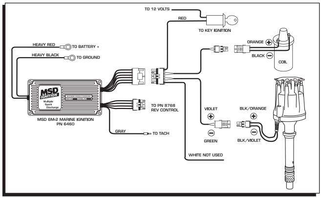
Figure 11 Wiring to an MSD 6M-2 Ignition Control.
