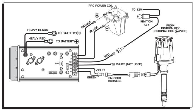
Figure 12 Wiring to an MSD 7ML-2 Ignition Control.
