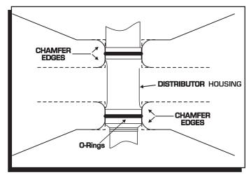
Figure 10 Modified Chevy Block for use with O-Rings.
