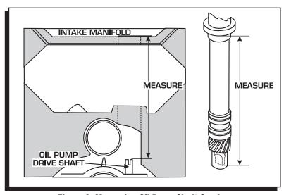
Figure 8 Measuring Oil Pump Shaft Overlap.
