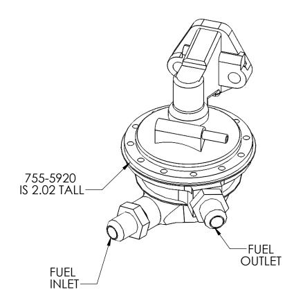
INSTALLATION INSTRUCTIONS: 1) REMOVE THE STOCK BOTTOM UNIT FROM THE FUEL PUMP. 2) MAKE SURE THE BLACK DIAPHAM IS NOT TORN AND BRITTLE. IF SO THE UPPER UNIT WILL NEED TO BE REPLACED. 3) SLIDE THE STOCK UPPER UNIT ON TO THE NEW LOWER UNIT. SOME PUMPS, LIKE SHOWN, WILL ALLOW THE UNIT TO BE CLOCKED TO HELP WITH FUEL LINE PRUMBING. 4) APPLY RED LOCTITE TO SCREWS AND TORQUE TO 40 INCH LBS.. 5) BOTH THE FUEL INLET AND **OUTLET HAVE -8 AN FITTINGS.**
