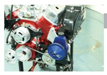
If using the plastic housing pump mounts it directly to the bracket using the 5/16" tapped hole and the slot closest to the engine.
