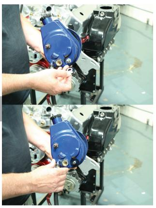
Put the pump on the bracket using the 3/8" hole and slot at the end of the bracket.
