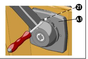
2 Adjust throttle lever friction turning on screw (21) with a Phillips head screwdriver (clockwise to increase and counterclockwise to decrease the friction). When adjustment is ended, close the drilled hole by inserting the provided screw cover (P).
