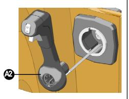
2 Attach the lever unit using screw (M) and press on cap (N).
