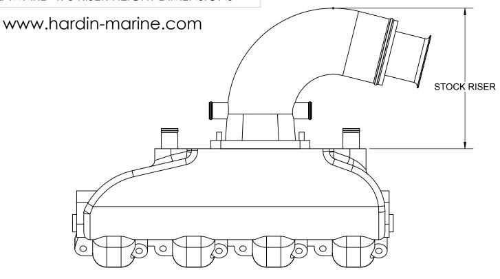
MEASURE FROM RISER FLANGE TO TOP OF RISER AS SHOWN. THE CHART BELOW SHOWS THE MERCURY HEIGHT AND THE SEAWARD KIT TO ORDER.
