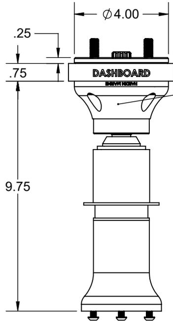
THE STEERING COLUMN BEZEL ALLOWS THE COLUMN TO BE USED UP TO A 1-1/2 THICK DASHBOARD.
