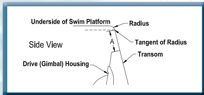
NOTE: When measuring distances on a built in swim platform, measure to the tangent of the radius as shown in the illustration to the right. >
