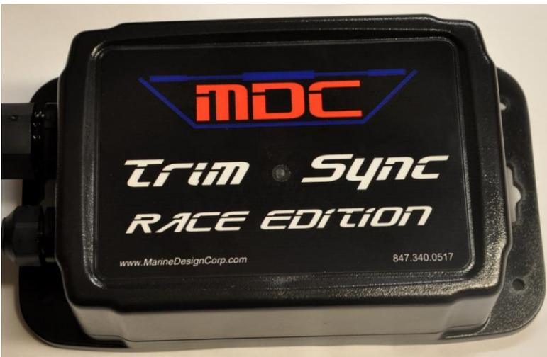
TrimSync monitors the trim for twin and triple engine boats, so when the operator presses the BOTH/ALL button, it will automatically adjust the drives / outboards to be in perfect alignment, *every time*. You will never have to worry about how accurate your mechanical trim indicators are because TrimSync will always move the slowest drive / outboard to match the others. TrimSync is compatible with all LED and electronic trim indicators. In
