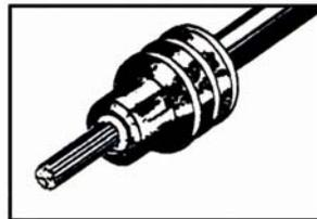
2. Align seal with cable insulation.
