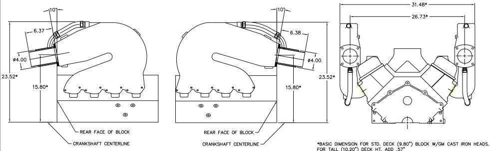
\*BASIC DIMENSION FOR STD. DECK (9.80") BLOCK W/GM CAST IRON HEADS. FOR TALL (10.20") DECK HT. ADD .29" FOR DART 360 HEADS ADD .27" FOR DART 360SR HEADS ADD .44"
