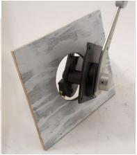
After making sure the plate is straight and level mark the 4 holes thru the outer plate and drill using a 1/4" drill bit.
