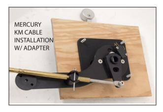
The cable can enter from the rear, front, or the bottom of the shifter and push or pull the cable from these installation points. See pictures below. (Note: Use loctite on all mounting screws to prevent them from coming loose during operation)
