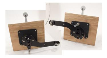
The 33c cable will use the rod end attached to the shift arm and the clamp on the pivot disc then just adjust as needed for smooth gear operation.
