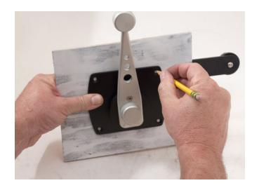
Now slide the rear retaining plate on the back side of the panel and install using the 4 counter sunk screws removed in a previous step. Tighten until the shifters inner and outer plates are pulled tight to the panel.
