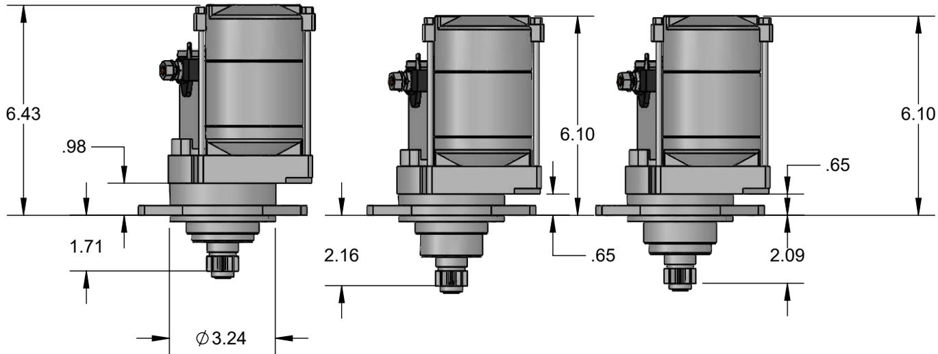
YOU MUST HAVE A MINIMUM .04 BETWEEN RING GEAR AND PINION GEAR
