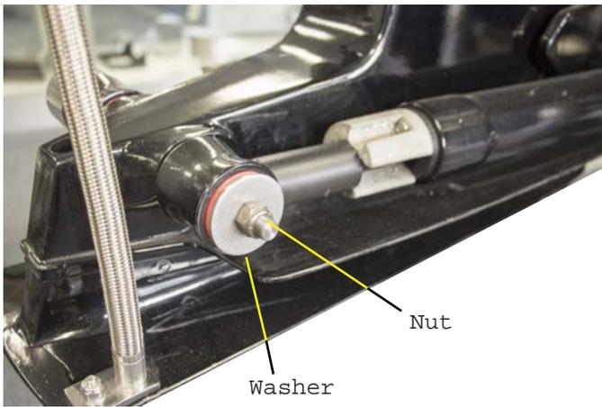
2. Install trim pin cup on trim pin and secure with nut. Tighten nut until approximately 2 threads are exposed through nut. Do not over tighten nut, as rubber bushings may be damaged.
