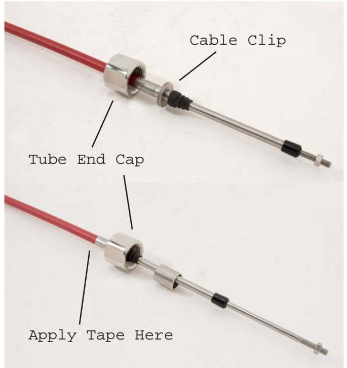
4. Install spring spacer onto cable and slide into end cap until it butts against cable clip. Extend cable fully.
