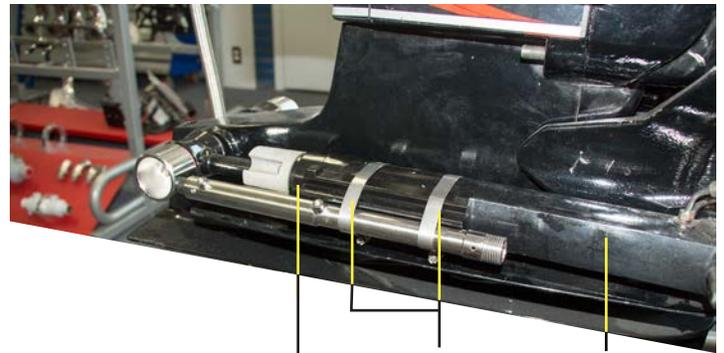
Preform Clamps over actuator tube in areas shown for ease of installation.
