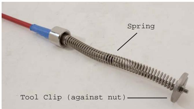
7. Thread push rod onto the cable end until it contacts the cable nut. Remove tool clip so spring contacts push rod.
