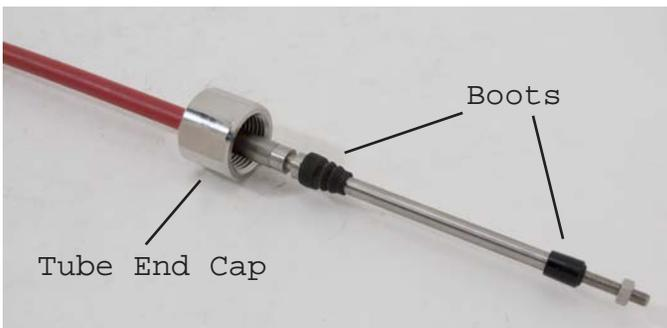
3. Install cable clip into cable groove. Slide tube end cap over cable clip and secure to the cable with tape.
