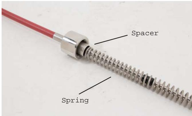
6. Compress spring and install tool clip between spring and cable nut. Slowly release tension on spring until it holds tool clip in place.
