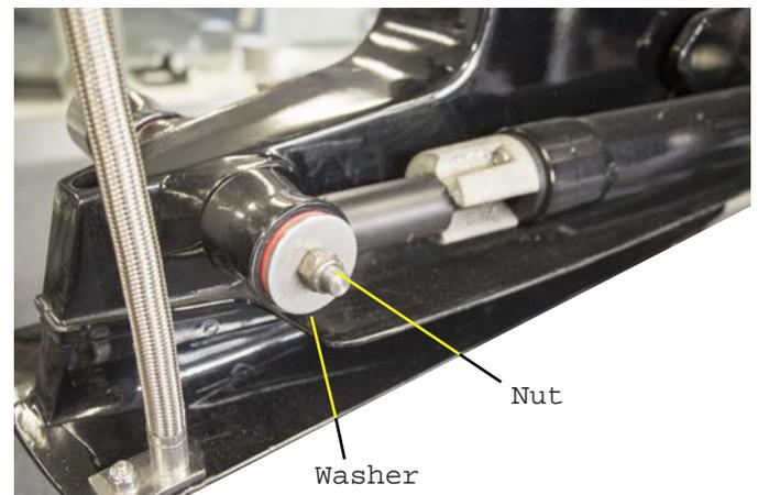
2. Install trim pin cup on trim pin and secure with nut. Tighten nut until approximately 2 threads are exposed through nut. Do not over tighten nut, as rubber bushings may be damaged.
