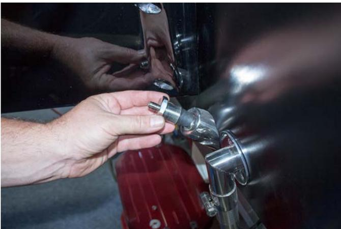
12. Push the 3 sensor wires through the fitting and into the boat until the cable nut can be threaded onto the fitting and then tighten.
