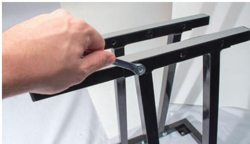
7) Install bolts with the button head on inside.
