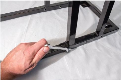
4) Install bolts with the button head on inside.
