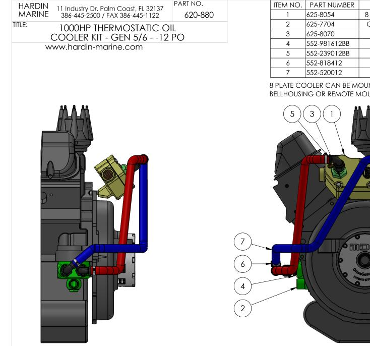
ITEM NO. PART NUMBER DESCRIPTION QTY. 8 PLATE BRAVO COOLER HOUSING 1 GEN 5/6 THERMOSTATIC ADAPTER 1 FITTING, -12 AN OIL COOLER 2 FITTING, 3/4NPT x -12 2 4 HOSE END, -12 90 DEG. CLAMP, -12 PUSH LOC 4 -12 PUSH ON HOSE 8
