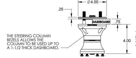
THE STEERING COLUMN POSITIONS THE STEERING WHEEL MOUNTING FACE 4" AWAY FROM DASHBOARD, BASED ON 3/4 DASHBOARD THICKNESS. FOR ADDITIONAL SIZES, HARDIN ALSO SELLS 137-9121 6" COLUMN AND 137-9122 8" COLUMN.
