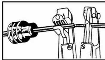
1. Apply seal to cable, before stripping insulation.
