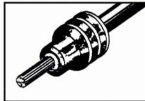
2. Align seal with cable insulation.
