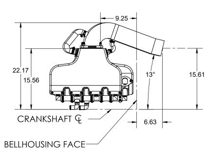
CAUTION\*\* HARDIN MARINE MANIFOLD SYSTEMS ARE DESIGNED FOR USE ON ENGINES WITH FULL TIME CONSTANT WATER CIRCULATION AT ALL TIMES. NOTE\*\* AFTER APPROXIMATELY 2-5 HOURS USE OR NUMEROUS ENGINE HEAT CYCLES ALL HARDWARE MUST BE RETORQUED AND OR TIGHTENED.
